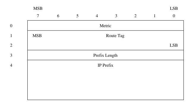
Metric is an integer 1-15 as used in RIP. 1 identifies a directly connected network and higher values indicate number of hops or other weighting.
